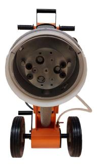
Machine in maintenance position - underside of the grinding head is accessible
