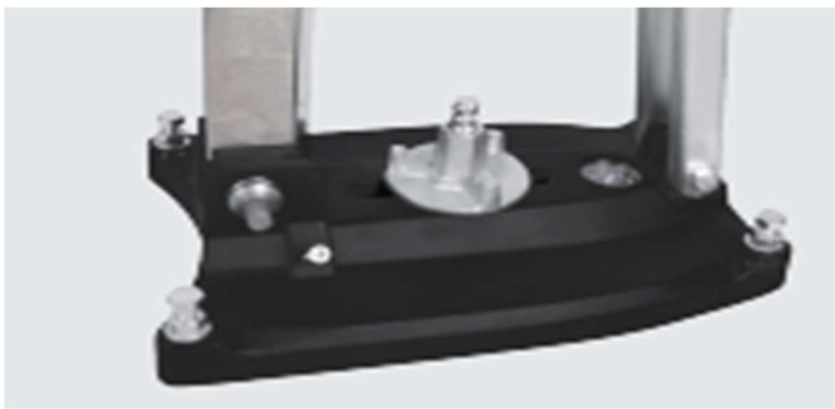
Base plate of the core drilling rig secured with cord threaded rod and wing nut
