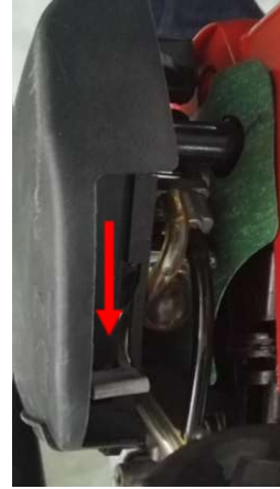
Start flap open (Start flap lever downwards)
