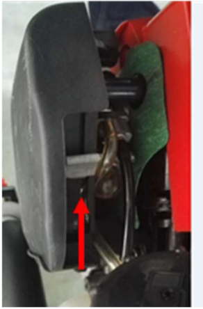
Start flap closed (Start flap lever upwards)
