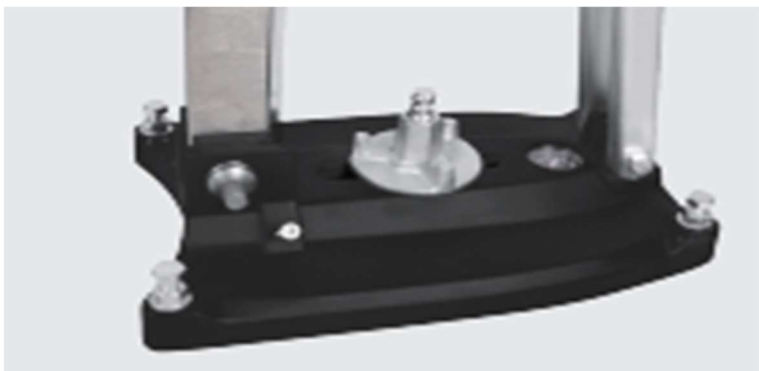
Base plate of the Core drilling rig fastened with threaded rod and disc wing nut
